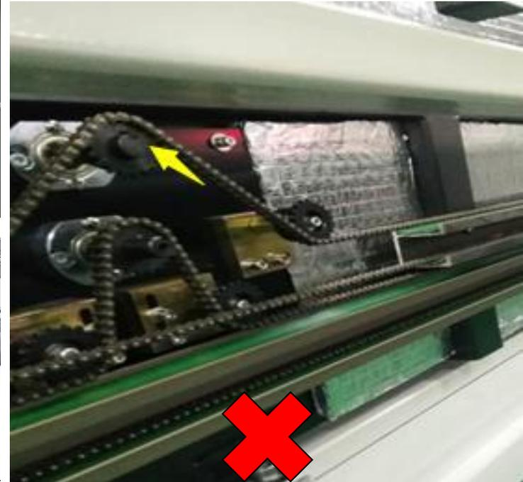
Other company design (Chain drive, poor synchronization, inconsistent width, easy to jam PCB)
