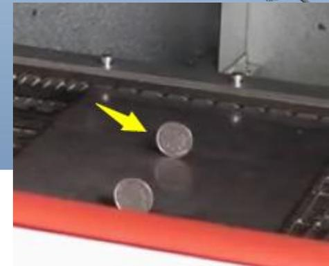
**Guide Rail will not deformed!!!**
