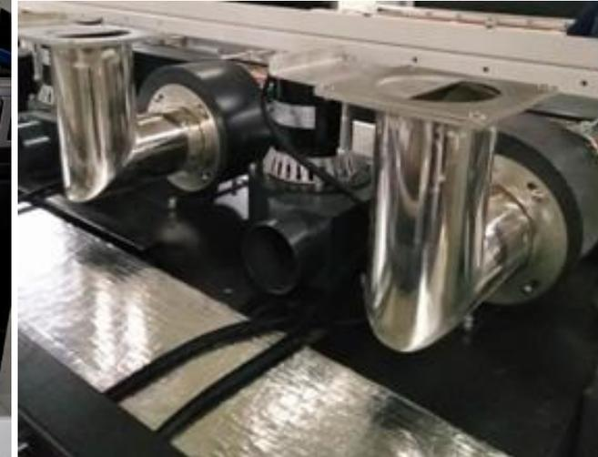
ETA cooling system is more reasonable, water cooling and air cooling can be replaced at any time, and nitrogen in the cooling zone can be monitored
