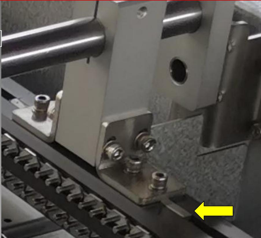
ETA guide rail adopts non-destructive design without damaging the guide rail body, and the link adopts positioning pin. Easy to maintain, no deformation.
